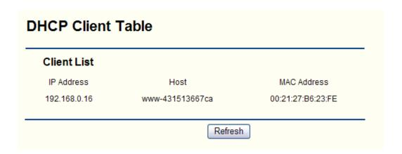
IP Address-The IP Address that the router has allocated to the DHCP client host.
