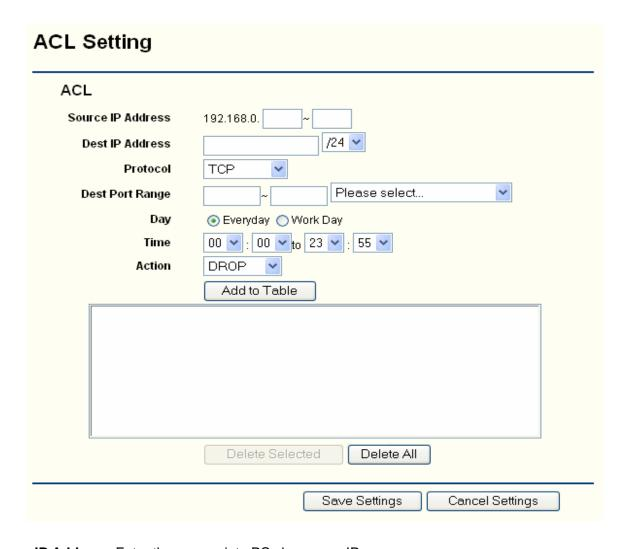
**Source IP Address**: Enter the appropriate PCs by source IP range.
