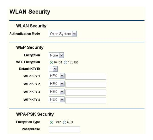
**Authentication Mode** – You can select desired Authentication Mode: Open System, Shared, WEP Auto, WPA-PSK and WPA2-PSK. When you select Open system or Shared or WEP Auto, you can set the WEP encryption. When you select WPA-PSK or WPA2-PSK, you can set the WPA-PSK Security.
