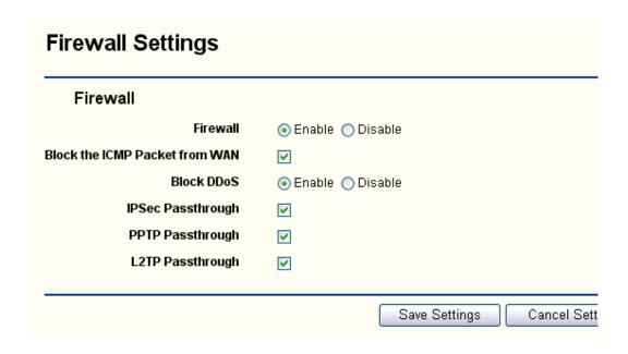
**Firewall** – the general SPI firewall switch is on or off.
