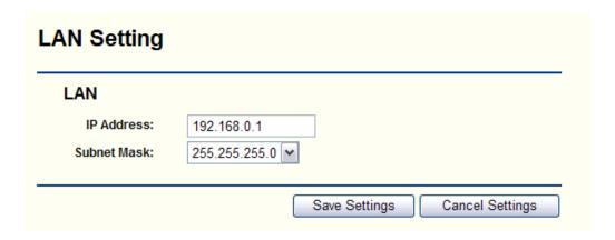
IP Address-Enter the IP address of your router in dotted-decimal notation(factory default 192.168.0.1)
