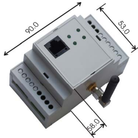
Picture 1. External view and measurements of the device
